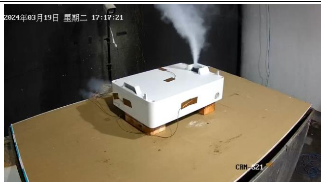
Figure 5: During thermal runaway (Time in 17:17)
