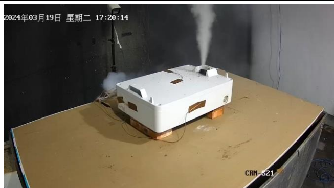
Figure 7: During thermal runaway (Time in 17:20)
