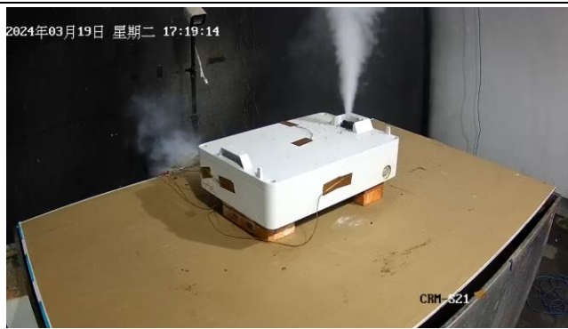
Figure 6: During thermal runaway (Time in 17:19)
